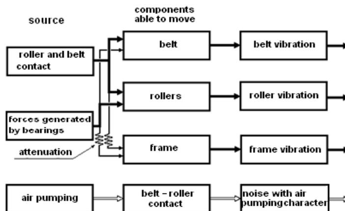
Fig. 1. Noise generating mechanisms of the conveyor belts
