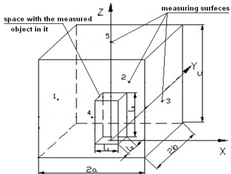
Fig. 2. Test arrangement for measurements conducted in an enclosed space
