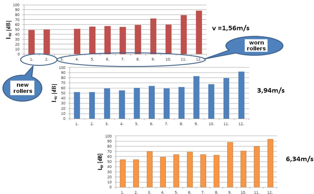
Fig. 5. Noise output levels measured in the case of the individual rollers
